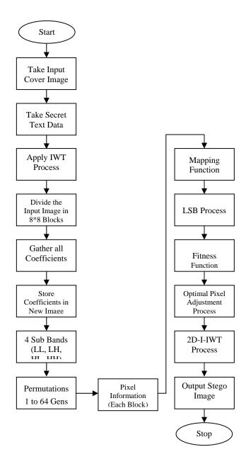
Fig.6 Flow Chart of the Data Embedding process
