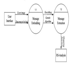
Fig. 2 Level 1 DFD of Proposed Steganography Model
