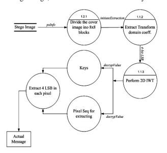
Fig. 4 Level 2 DFD of Proposed Steganography Model
