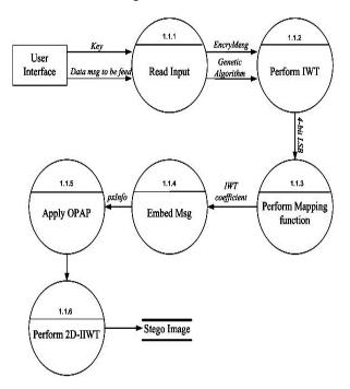
Fig. 3 Level 2 DFD of Proposed Steganography Model
