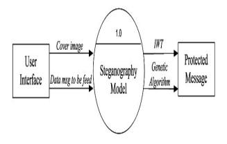
Fig. 1 Level 0 DFD of Proposed Steganography Model
