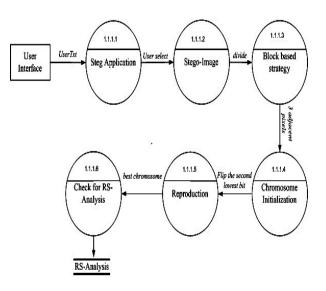
Fig. 5 Level 3 DFD of Proposed Steganography Mode
